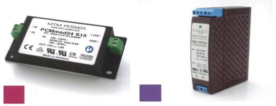
**PMmed** / **PCMmed** encapsulated designs for medical applications are available in power ranges of from 15 watts -100 watts. The primary voltage range of 90 -264 Vac / 100 -353 Vdc with single output selections for PCB and chassis mount applications where EN/UL 60 601-1/EN/UL 60 950-1 ( $2^{nd}$  Edition) is necessary.
